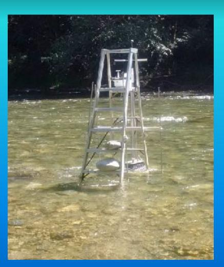
DIDSON located on ladder in the river, with computer recording data on bank – at Parker Jefferson's
