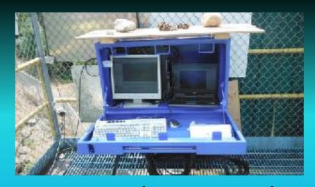
Locked in 'secure' boxes, DIDSON records constantly (weir), video records motion events (fishway)
